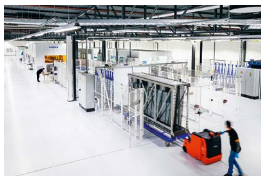
Production of liquid crystal window modules in Veldhoven, the Netherlands.
